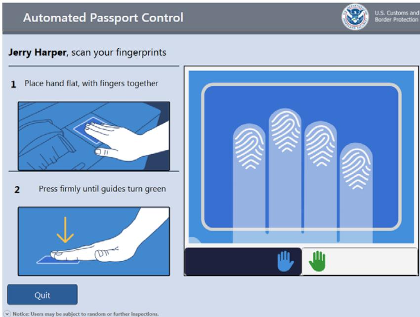
9 The kiosk provides white, yellow, and green indicators for each finger to provide the traveler with feedback on how well the fingerprints are being read:
