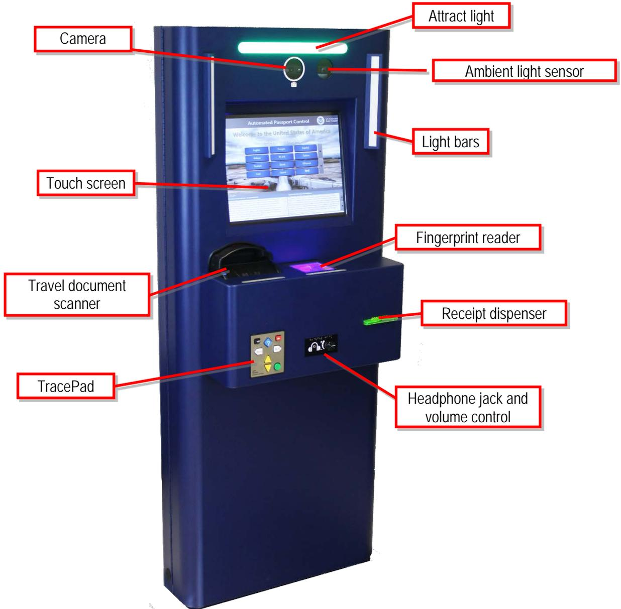
Figure 1: Standard Kiosk Components
