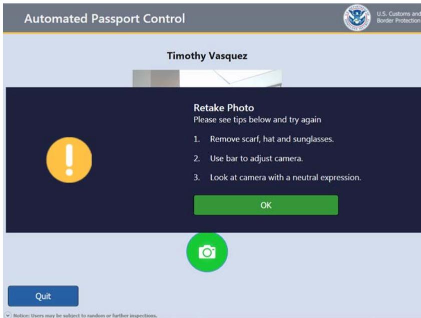
The above screen displays if the traveler's photo is invalid during the photo capture process.
