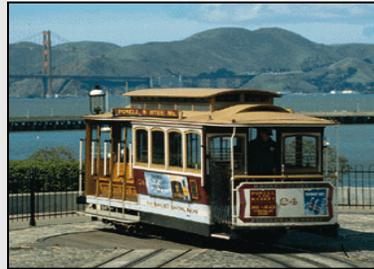
A railway propelled by moving cables located beneath the street. While popular at the turn of the last century, the only surviving system is operated in San Francisco.
