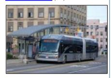
Fixed-route bus systems that combine passenger stations, traffic signal priority or pre-emption, low-floor vehicles or level-platform boarding, and separate branding of the service. This is often a lower-cost alternative to light rail.
