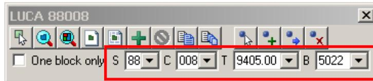
Click on the **Pick Block**
