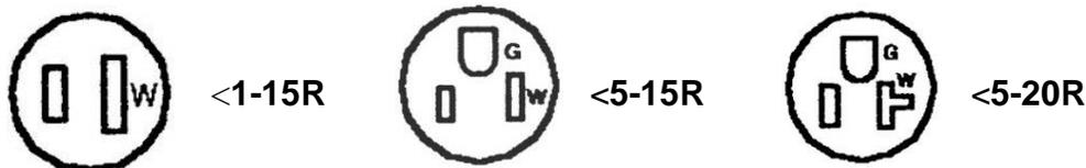
**Figure 5-NEMA Receptacle Configurations (found in typical household use)**
