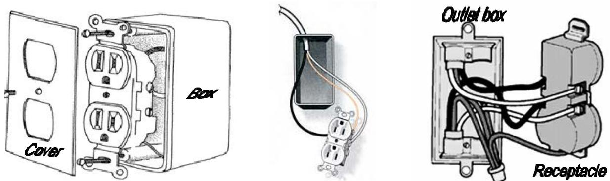
**Figure 3 - Outlet Boxes with Installed Grounded Receptacle**
