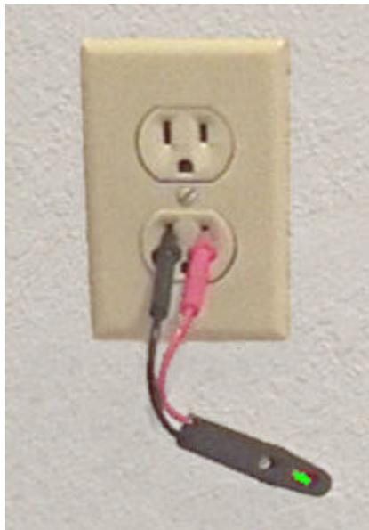
Insert one probe of the circuit tester into the small slot and the other probe into the large probe. If the circuit tester lights up, you have power to the outlet. Now place one probe in the small slot and the other probe into the "U" shaped ground hole. The indicator should light up if the outlet is grounded. Test both outlets because they can be wired separately. The fact that one is properly wired does not guarantee that they are both properly wired.
