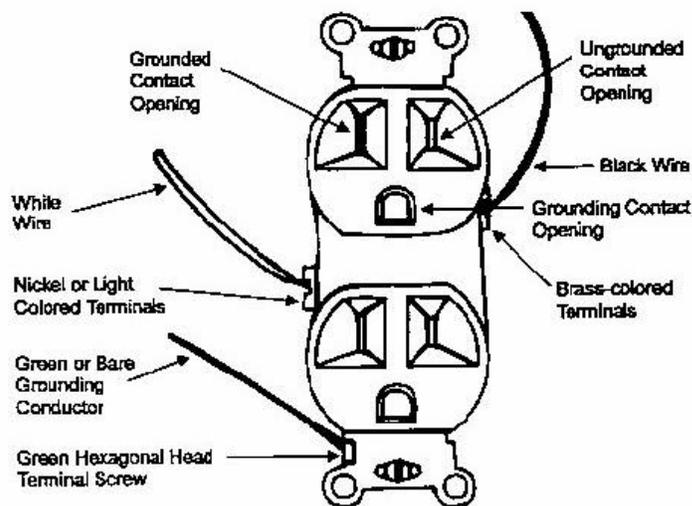
**Figure 1 - Side-wired Grounded Duplex 15A Receptacle (front view)**
