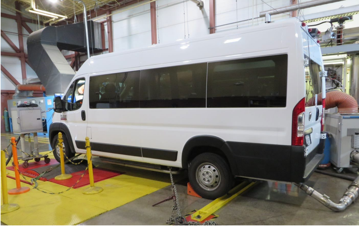
BUS TESTED ON CHASSIS DYNAMOMETER FOR PERFORMANCE, FUEL ECONOMY AND EMISSIONS
