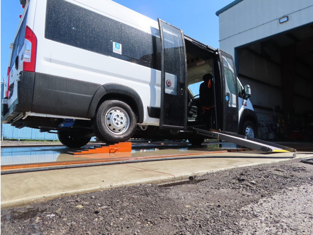
RIGHT REAR WHEEL SIX INCHES HIGHER
