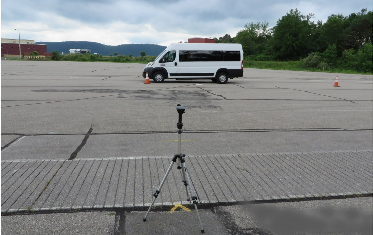
TEST BUS UNDERGOING EXTERIOR NOISE TESTING
