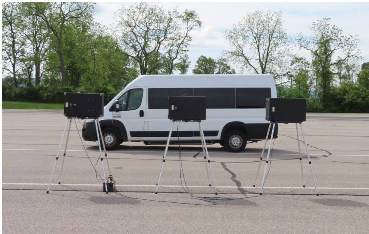
TEST BUS SET-UP FOR 80 dB(A) INTERIOR NOISE TEST
