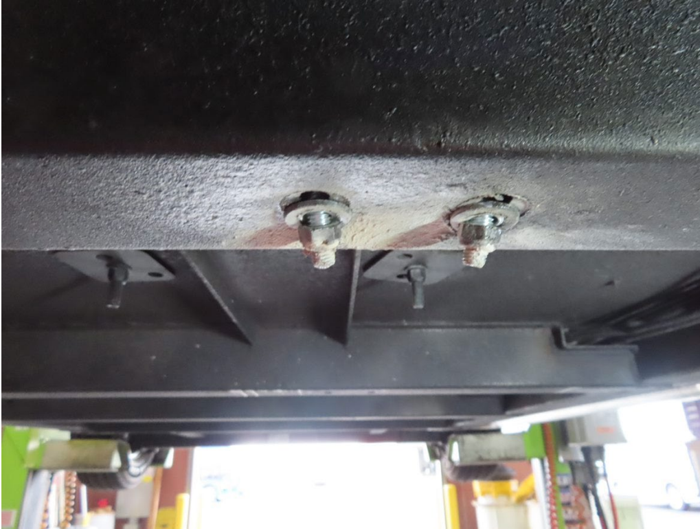
TWO BACK BOLTS ON ADA GATE LOCKING PLATE ARE BENT FROM HITTING ON DURABILITY TRACK (53 TEST MILES)
