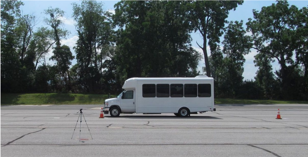
TEST BUS UNDERGOING EXTERIOR NOISE TESTING
