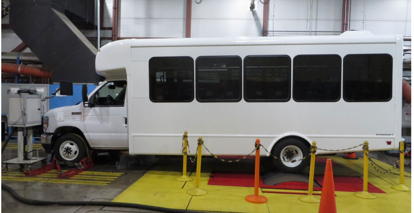
BUS TESTED ON CHASSIS DYNAMOMETER FOR PERFORMANCE AND FUEL ECONOMY
