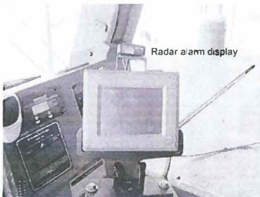
Figure 7. Preco radar alarm display mounted in truck cab.
