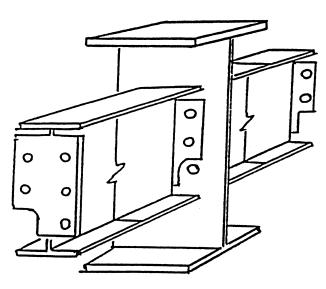
Clipped end connections are connection material on the end of a structural member which has a notch at the bottom and/or top to allow the bolt(s) of the first member placed on the opposite side of the central member to remain in place. The notch(es) fits around the nut or bolt head of the opposing member to allow the second member to be bolted up without removing the bolt(s) holding the first member.
