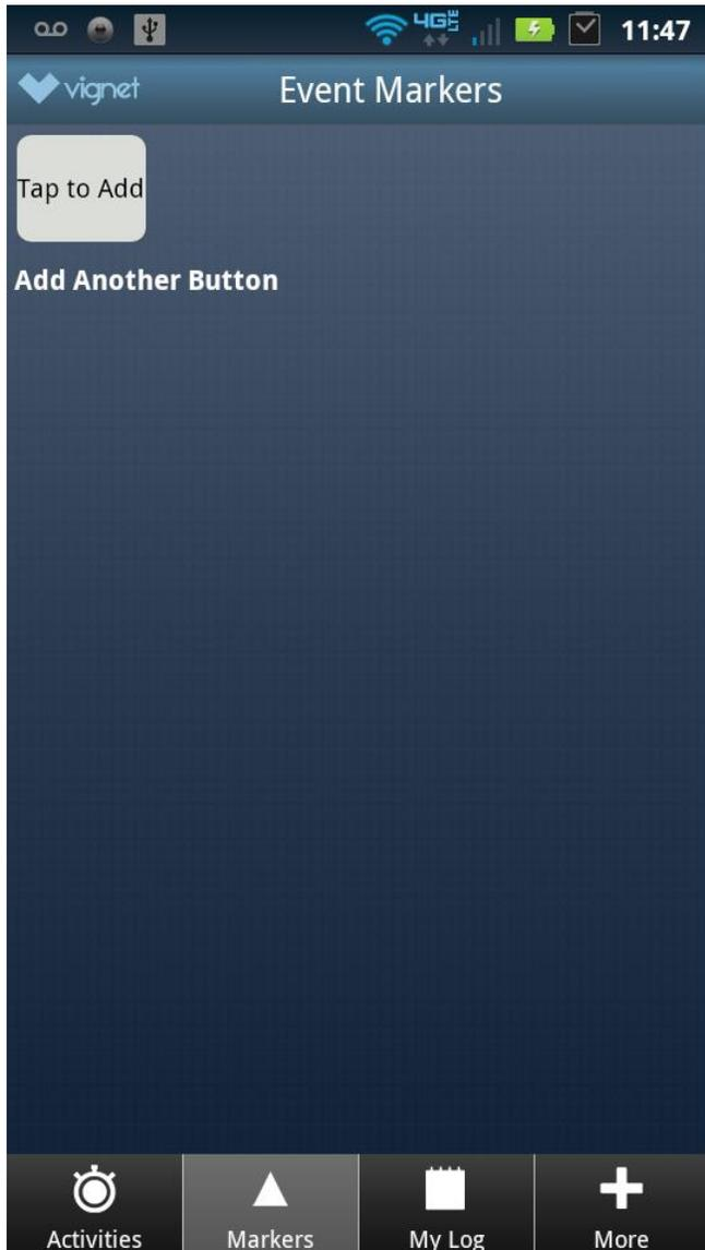
Description: To customize a Marker button, the user begins from the Markers screen and taps on the button which displays “Tap to Add”, in order to add additional buttons to the screen the user pressing the “Add Another Button” link.
