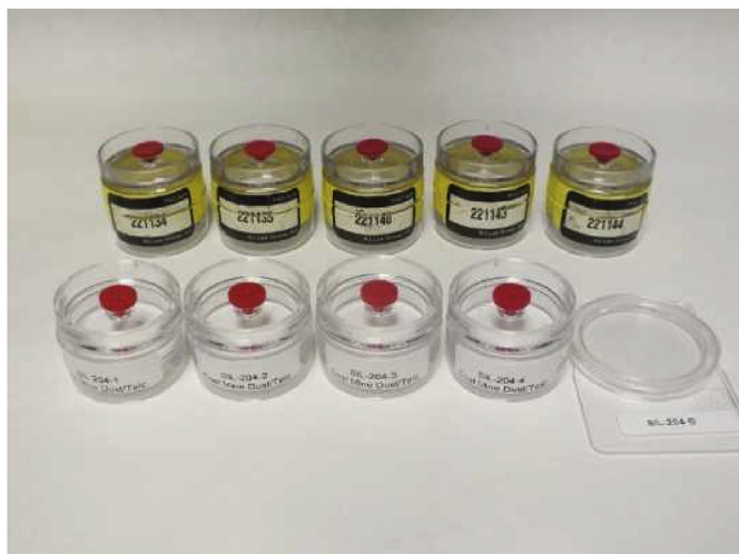
Fig. 2. Real-world (back row) and AIHA-prepared (front row) filters sent to laboratories for analysis.
