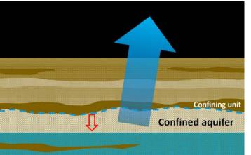
**#7** Aquifer compaction after aggressive dewatering Enbridge conducted aggressive dewatering in many places for a variety of reasons, e.g. aquifer breach responses, hillside destabilization response (Walker Brook), trench dewatering during construction, etc. Compaction of unconsolidated aquifers is likely, leading to permanent loss of water storage capacity and possible land subsidence.
