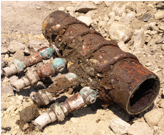
Corroded water main with lead fittings.
