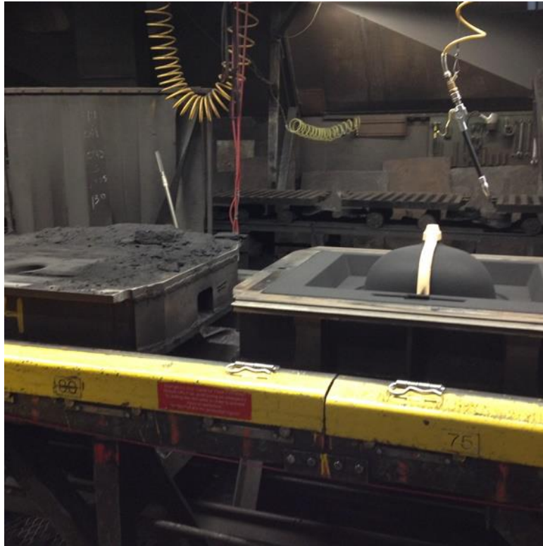
Cleaning Sand off Molds Prior to Closing
