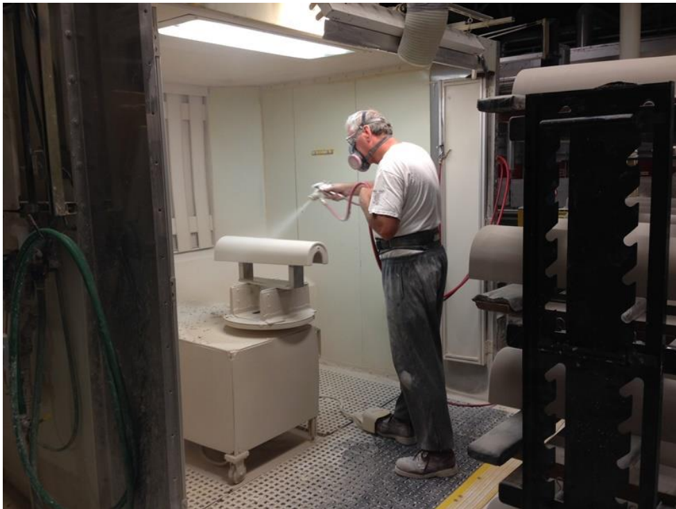
Cleaning Dry-Filter Glaze Spray Booths Where Glaze Overspray is Dried to the Booth Walls and Floors
