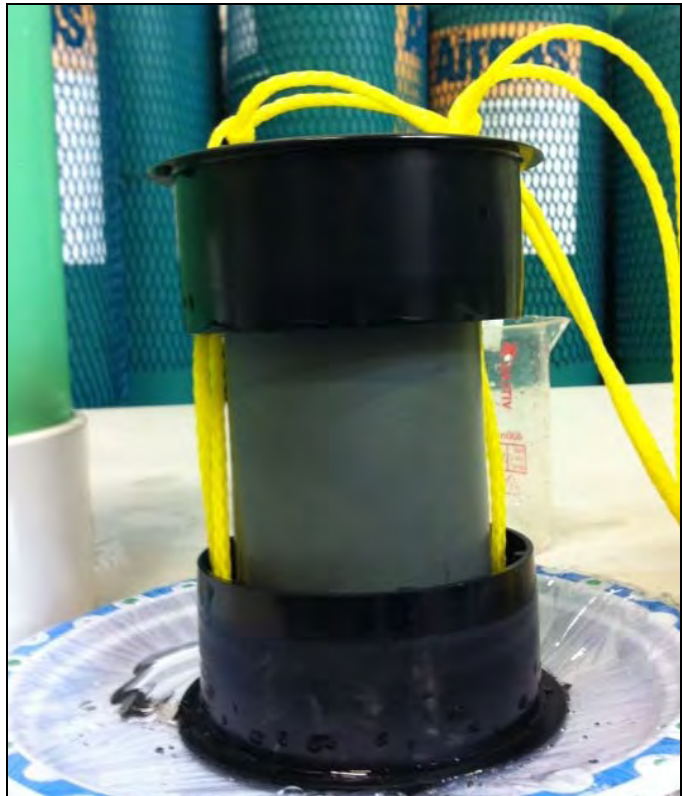
Figure 1. Tailings backfill sample cylinder (courtesy of WETLAB, Sparks, NV).
