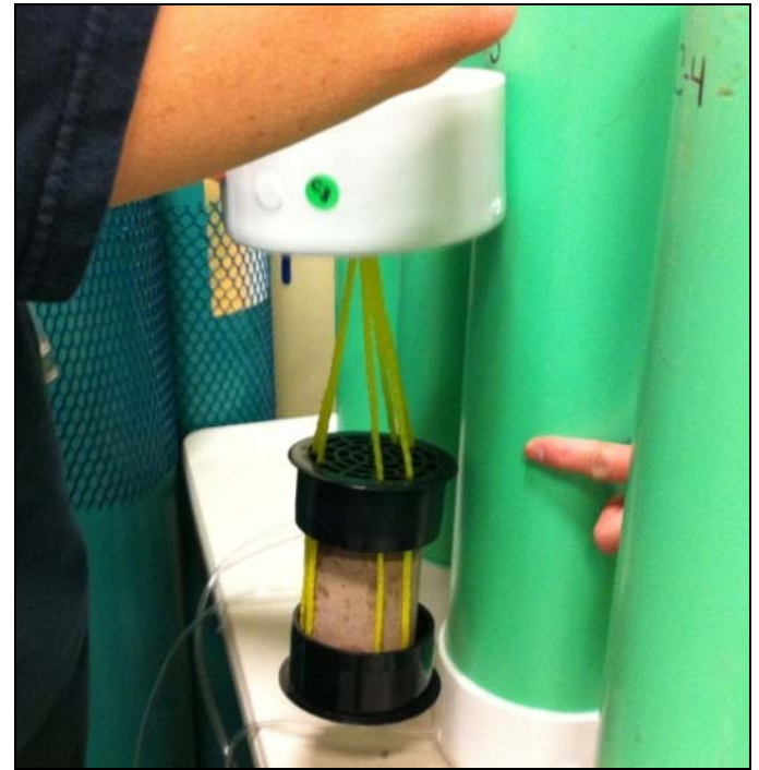
Figure 2. Transferring cylinders (courtesy of WETLAB, Sparks, NV).
