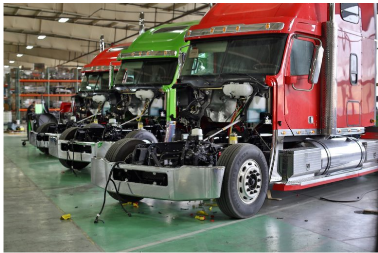
Fitzgerald Glider Kits receives cabs and chassis directly from Freightliner, Kenworth and Peterbilt, then installs remanufactured 2003 and older Detroit Diesel Series 60 engines and reman Eaton-Fuller transmissions. Glider assemblers like Fitzgerald will need to either bring these engines into compliance with 2010 regulations or seek alternative paths to ensure compliance with Phase 2 emissions regulations.
