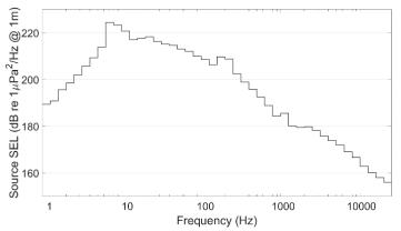
Figure B-2. Maximum directional source level (SL) in the horizontal plane, in each 1/3-octave-band, for the 4130 in<sup>3</sup> airgun array (1–25,000 Hz).
