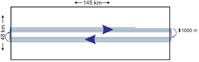
Figure 3. Simulated portion of the track for the 3-D NAZ seismic survey.
