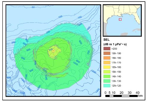
Figure 8. 4130 in<sup>3</sup> airgun array at the Central-Slope region (Site CM3), Season 3 (September): Broadband (10–5,000 Hz) maximum-over-depth per-pulse SEL field. Blue contours indicate water depth in meters.
