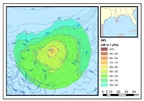
Figure 10. 4130 in<sup>3</sup> airgun array at the Central-Slope region (Site CM3), Season 3 (September): Broadband (10–5,000 Hz) maximum-over-depth SPL field. Blue contours indicate water depth in meters.
