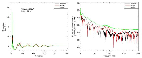
Figure B-1. The 4130 in<sup>3</sup> array: Predicted (a) overpressure signature and (b) power spectrum in the broadside, endfire, and vertical directions. Surface ghosts (effects of the pulse reflection at the water surface) are not included in these signatures as they are accounted for by the MONM propagation model.
