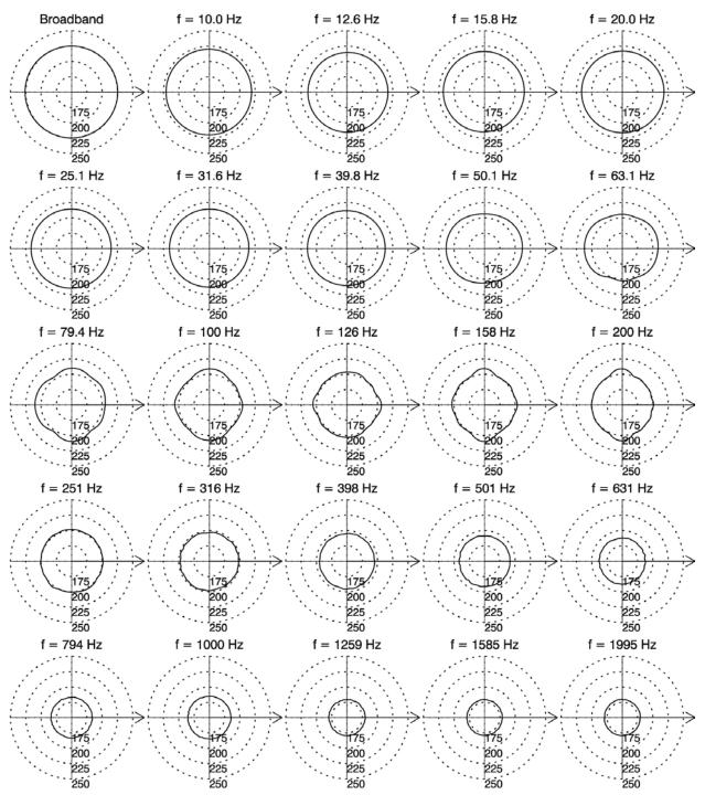
Figure B-3. Horizontal directivity of the 4130 in<sup>3</sup> array. Source levels (SLs, dB re 1 µPa<sup>2</sup>·s) in 1/3-octave-bands. The 1/3-octave-band center frequencies are indicated above each plot.
