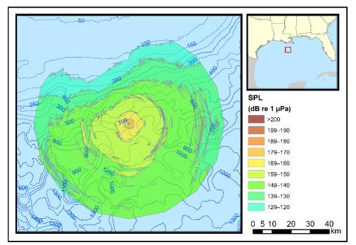
Figure 9. 4130 in<sup>3</sup> airgun array at the Central-Slope region (Site CM3), Season 1 (February): Broadband (10–5,000 Hz) maximum-over-depth SPL field. Blue contours indicate water depth in meters.
