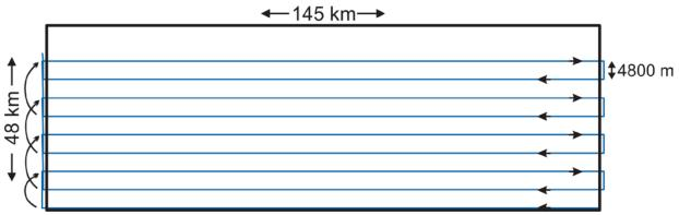
Figure 2. Simulated portion of the track for the 2-D seismic survey.
