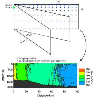
Figure C-3. The *N*×2-D and maximum-over-depth modeling approach.
