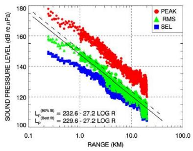
Figure C-1. Field measurements of peak and root-mean-square (rms) sound pressure level (SPL) and sound exposure level (SEL) versus range from a 20 in<sup>3</sup> airgun array. Solid line is the least squares best fit to rms SPL (Ireland et al. 2009).
