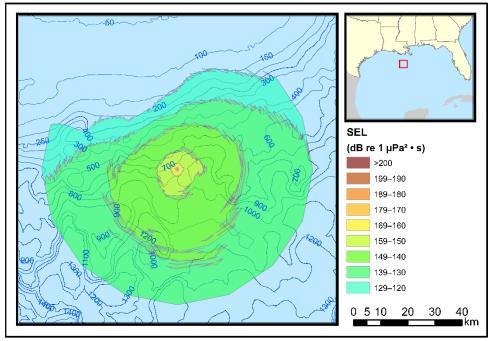
Figure 7. 4130 in<sup>3</sup> airgun array at the Central-Slope region (Site CM3), Season 1 (February): Broadband (10–5,000 Hz) maximum-over-depth per-pulse SEL field. Blue contours indicate water depth in meters.
