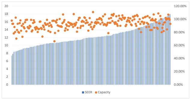
Each blue line below represents the SEER rating of specific retrofit units and the orange dot represents the corresponding, normalized capacity of that same unit.
