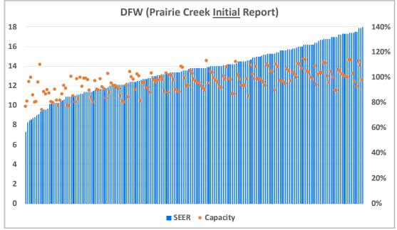
Each blue line below represents the SEER rating of specific retrofit units and the orange dot represents the corresponding, normalized capacity of that same unit.
