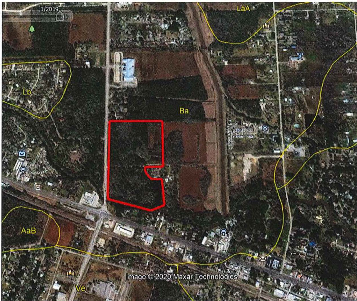
Figure 2. Soil map (Soil Web). Ba is the symbol for Bacliff clay, 0 to 1%, rarely flooded mapping unit. Note how well the different tonal patterns stand out on the subject property at this scale.
